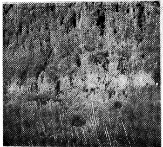
b.) Rod wear (150x) ( Subjective rating of "1")
